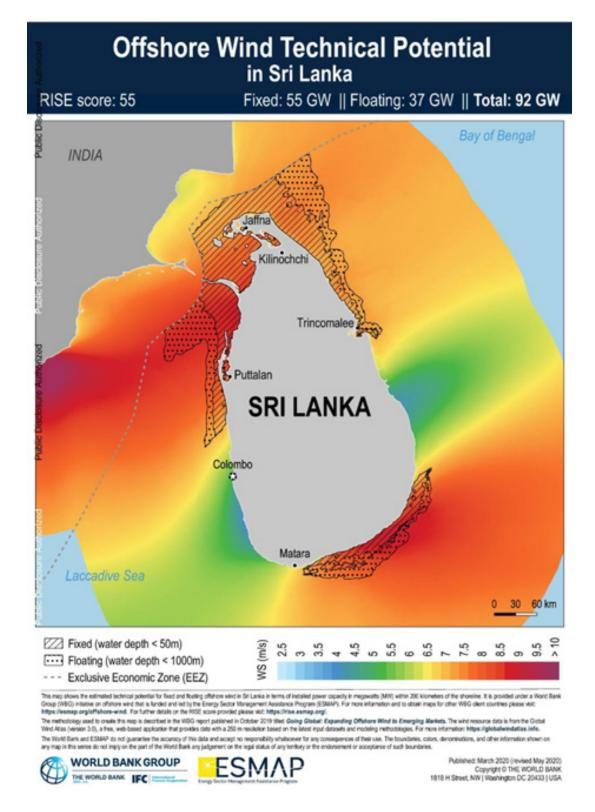
Figure 7: Offshore wind technical potential in Sri Lanka (World Bank, 2020)
